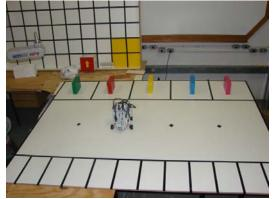
Fig. 6. FIONA at a random starting position. It then needs to learn the position of each group of cubes.
