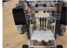
Fig. 1. Ramp inside the robot. The cube is dropped and carried on it.
