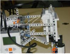
Fig. 3. Four-bar mechanisms and gears lifting claw.
