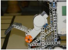
Fig. 5. Lock-gate that holds the cubes while FIONA moves.
